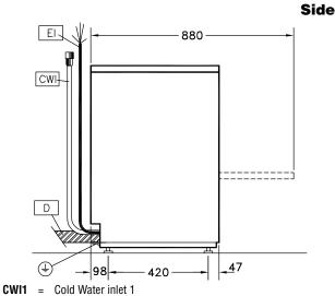
**Electrical Outlet** E0 WI Water inlet XR Rinse aid connection
